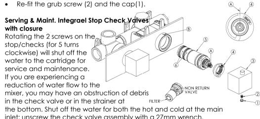
the bottom. Shut off the water for both the hot and cold at the main inlet; unscrew the check valve assembly with a 27mm wrench.
